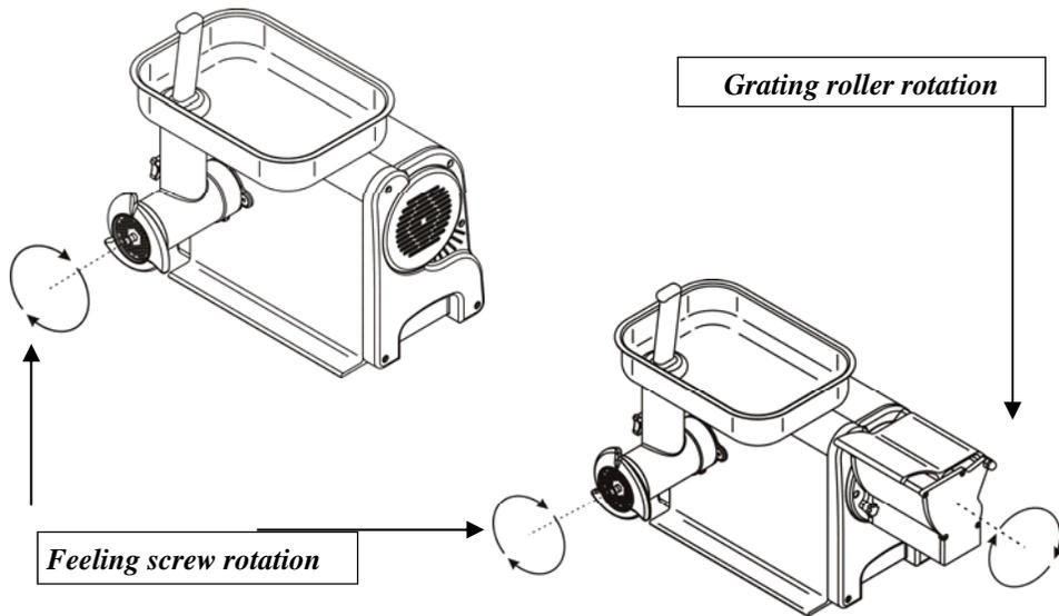
FIG. n°5 - Rotation sense of the feeding screw and of the grating roller
