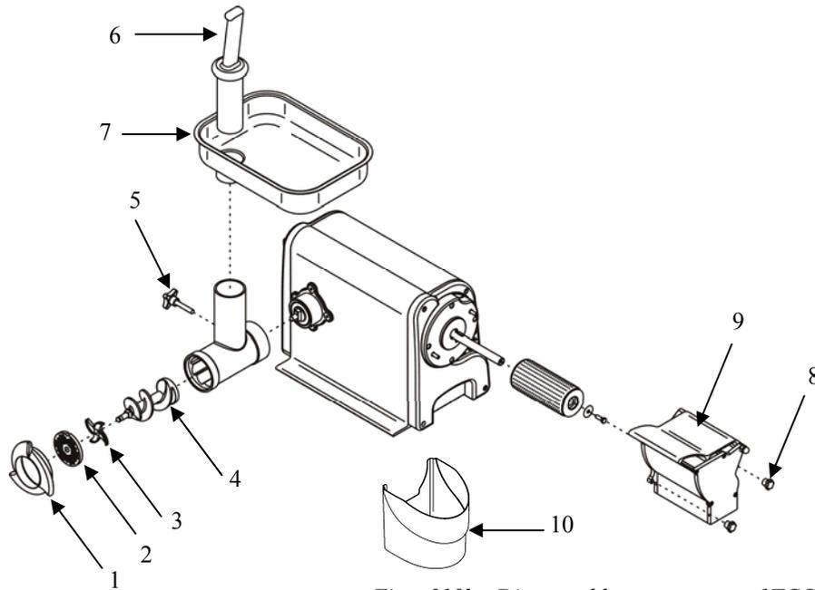
Fig. n°10b - Disassembly components of TCG
